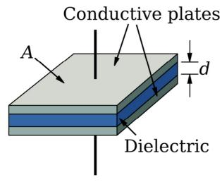
Capacitance is calculated by the above formula, in which k is a constant, A area, and d the distance between plates.
